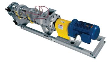
The material enters at one end of the cylinder and is whipped by the pins as it moves from the inlet through the shell and to the bottom outlets. As a fine spray of liquid is added at the entry section and distributed throughout the powder, fine mixing and micro-agglomeration will occur. The end result is a wetted, agglomerated and densified micro-pellet.
